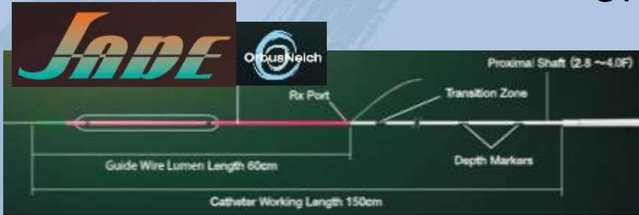
✓ “JADE is 0.014 compatible non-compliant balloon that has the longest guidewire lumen length (60cm) for strengthening pushability.”
